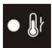
LED INDICATOR – OVERHEATING. Temperature inside charger exceed permitted value. Charging is off until temperature goes down. Restart of charging is automatic.
