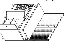
hauger boards, and into the side of SS Insert the Hexagon bolt with flange screw(M6X25) through the back of
